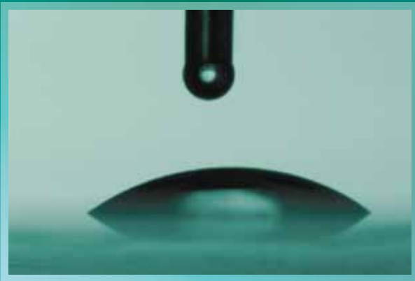
Low contact angle – high wettability
